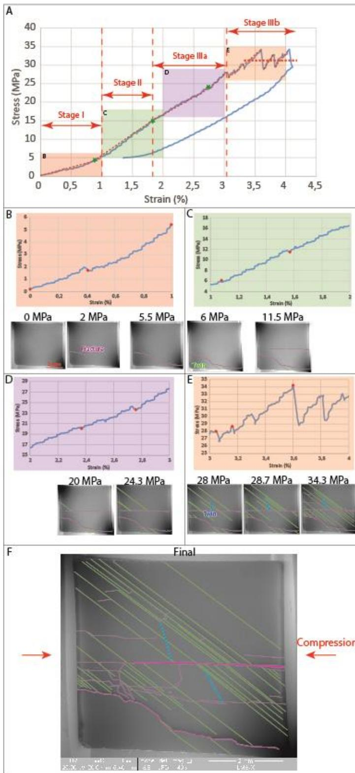
**Figure 2: Results from sample Pita. Stress (MPa) versus strain (%) curve showing the three stages described in the article. Each red point on the curves corresponds to one of the high-resolution pictures below. In the different pictures, the twin lamellae are in light green color. Fractures are in pink color.**
