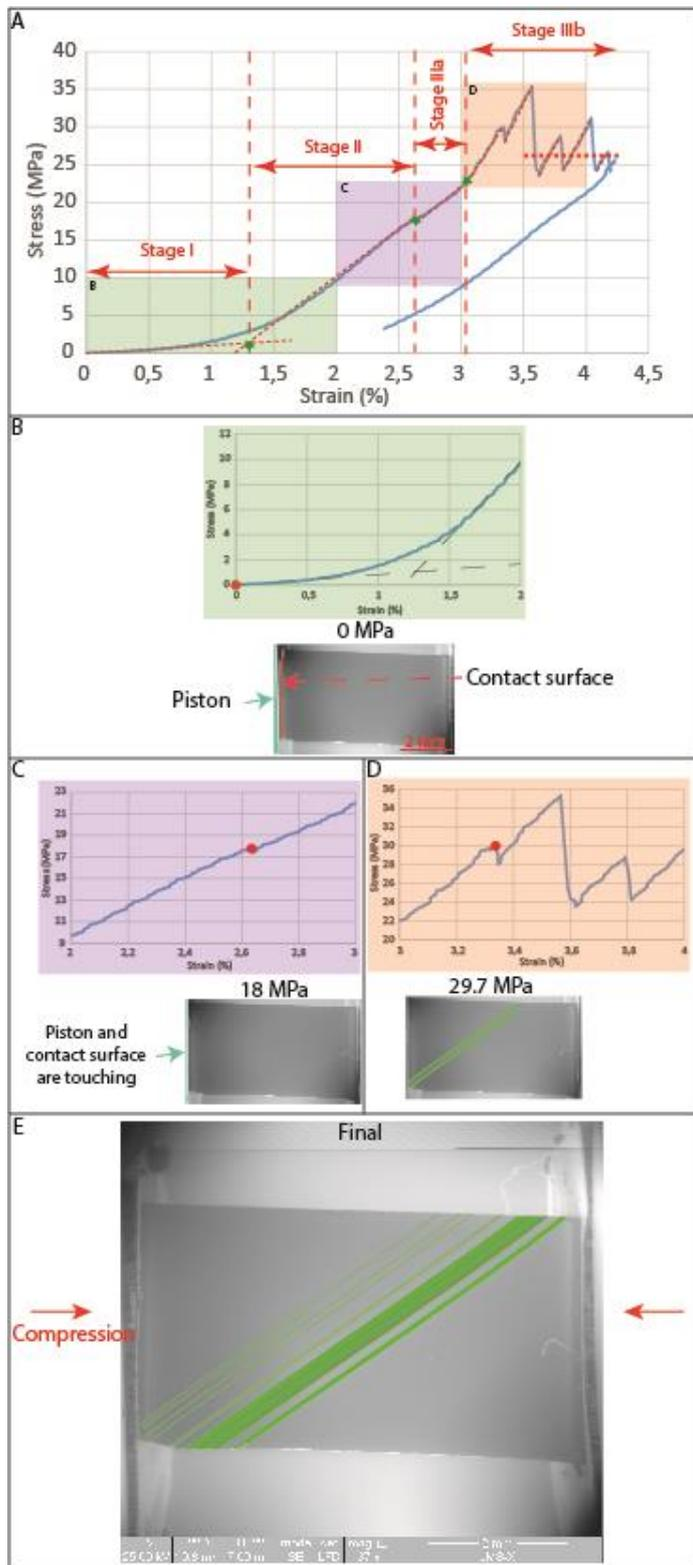
**Figure 3: Results from sample Johnny. Stress (MPa) versus strain (%) curve showing the three stages described in the article. Each red point on the curves corresponds to one of the high-resolution pictures below. In the different pictures, the twin lamellae are in light green color. Fractures are in pink color.**
