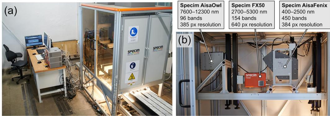
**Figure 4.** (a) Specim Sisurock hyperspectral drill core scanner with (b) mounted sensors in the visible to near-infrared and shortwave infrared (VNIR and SWIR), mid-wave infrared (MWIR), and longwave infrared (LWIR) range.
