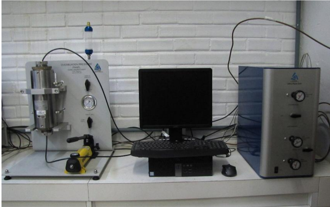
49 50 Figure S2. Ultra-Perm 610 gas permeameter with pressure sample saturator (Core Lab 51 Instruments).
