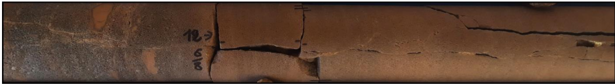
Structure vertical change as fonction of lithology, from cataclastic deformation band in very coarse sandstone to Mode I fracture in fine-medium sandstone from Tchirezrine II unit at Imouraren site
