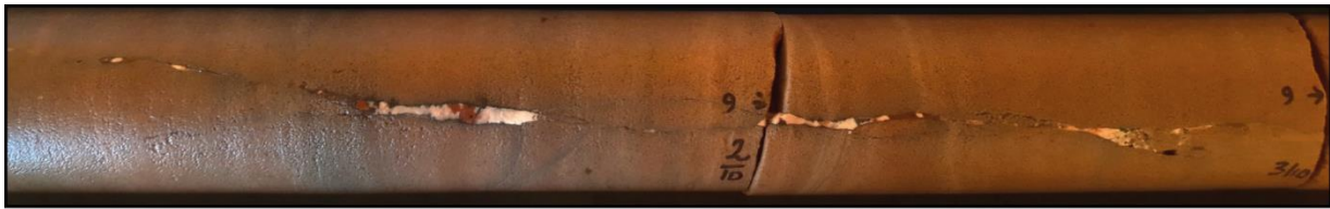
Mode I fracture with calcite seal in fine sandstone from Tchirezrine II unit at Imouraren site
