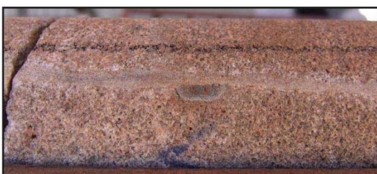
Cataclastic deformation bands crosscutting a clayey pebble from Tchirezrine II unit at Imouraren site (Orano Internal Report).
