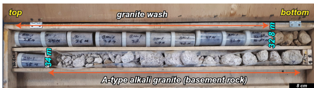
Figure D1. Photograph showing the drilled core. The lowermost part of the unconsolidated sediments, the granite wash, directly overlies bedrock. Cosmogenic ^{10}\text{Be} – ^{26}\text{Al} isochron dating samples are taken from this granite wash.
