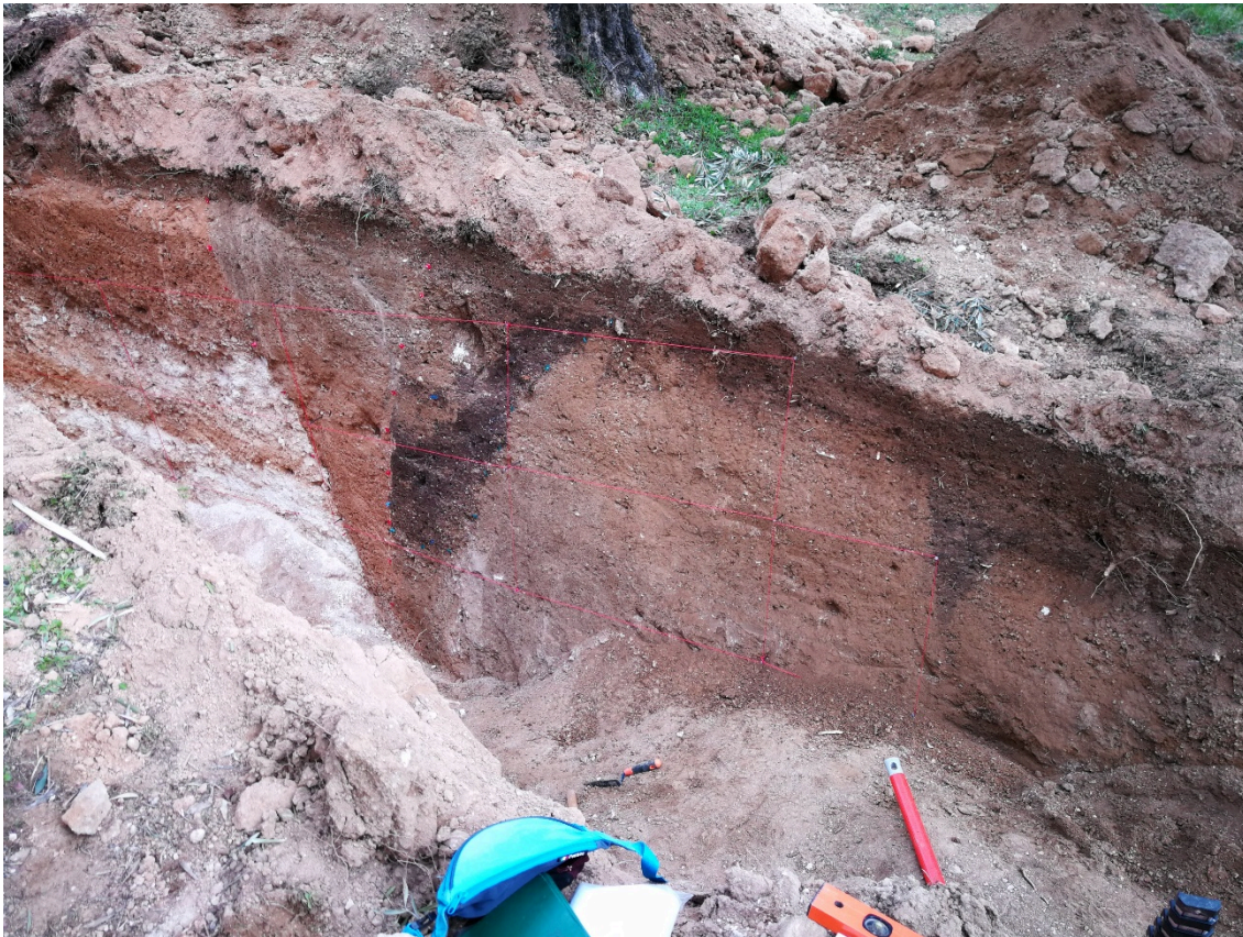
Figure S4. Southern wall of the trench TB. Detail of the FA and FB fault zones.
