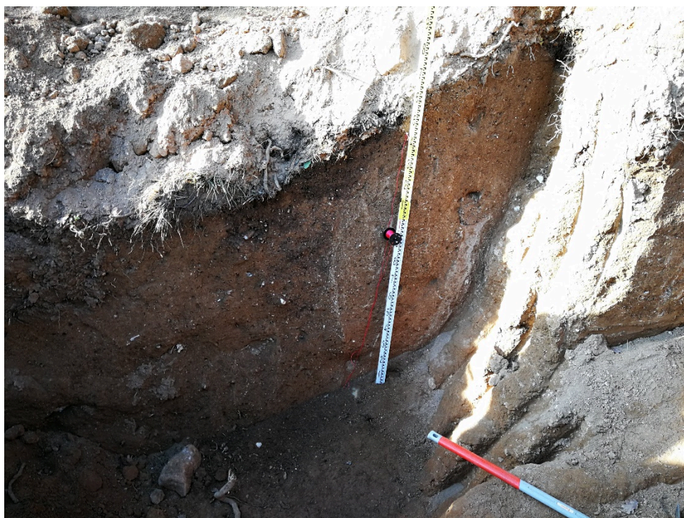
Figure S2. Northern wall of trench TA. Detail of the FA fault zone.
