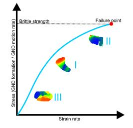
**Figure 15.** Schematic diagram for different finite crystal-plastic deformation patterns in zircon that are stress-strain rate dependent. I–III reflect deformation pattern types (I), (II) and (III), respectively. GND: geometrically necessary dislocations.
