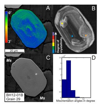
Figure 2. Grain BH12-01B\_29, no deformation-related lattice distortion observed. (a) EBSD map color-coded for zircon misorientation (blue-red:  $0-3^{\circ}$ ) of each pixel relative to a reference point (red star marker). (b) CL image with colored points representing relative degrees of crystallinity, measured by Raman spectroscopy. (c) EBSD pattern quality map; Ms: muscovite. (d) Histogram of the distribution of misorientation angles between neighboring data points.
