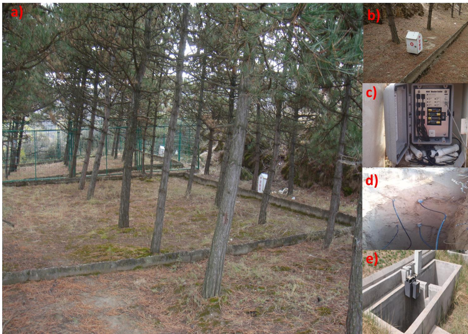
Figure S1 Take the pine trees plot as an example: a): the pine trees plot; b): the digital collection equipment (white box at the top of each plot); c) and d): 5 soil moisture and 5 temperature smart sensors were installed at 5 depths below the ground; e): the H-flume at the outlet of each plot.
