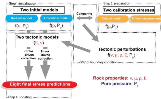
**Figure 3.** Flow chart detailing the different prediction strategies. See Sect. 3 for details. Rock properties used in the different models are  $\nu$  Poisson's ratio,  $\mu$  friction,  $\rho$  density, and  $E$  Young's modulus.
