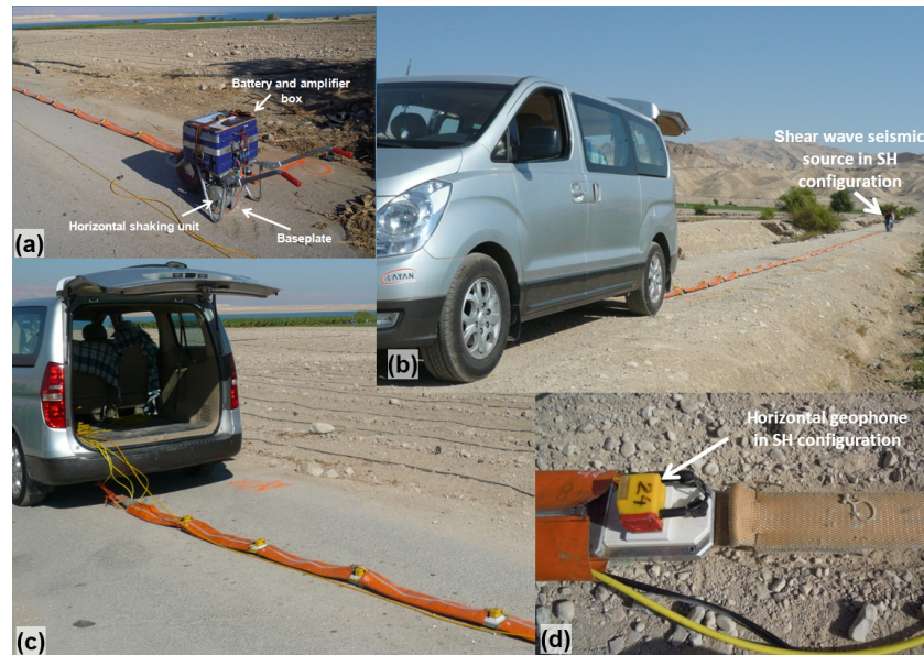
Figure 3. Photos of the shear wave seismic reflection acquisition campaign carried out in October 2013. (a) Wheelbarrow-mounted shear wave source system on asphalt pavement at start location of profile 2. (b) Recording car, towed land streamer and source during operation on profile 3. (c) Land streamer towed by the recording car during acquisition on profile 2. Colour paintings on the road surface were used for location numbering along the profiles. (d) Sledge-mounted horizontal geophone in SH (particle movement perpendicular to profiling direction) configuration along profile 3.
