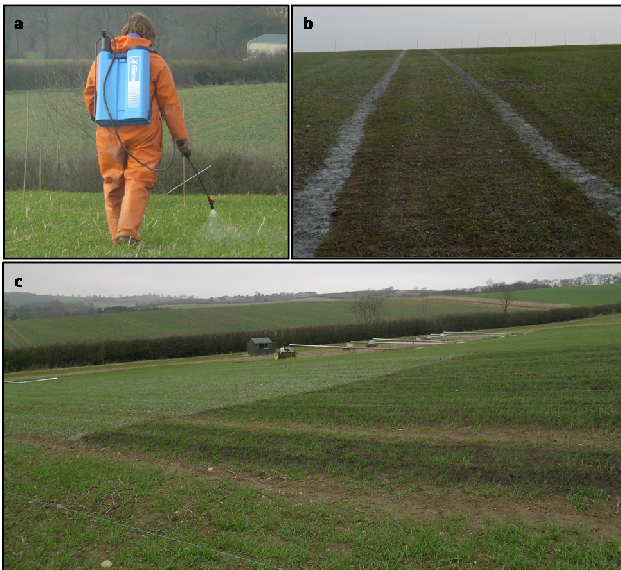
47 FIGURE S1. Spraying rare earth oxide (REO) powders onto the hillslope at Loddington in suspension using a 48 calibrated knapsack sprayer (a). REO tagged areas were clearly visible, for example \text{Nd}_2\text{O}_3 applied to the wheel 49 track areas (a), and \text{Pr}_6\text{O}_{11} on the midslope and \text{Sm}_2\text{O}_3 applied to the downslope areas (c).
