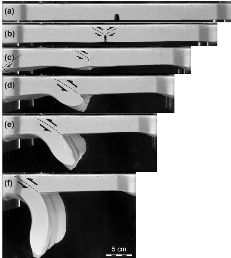
**Fig. 11.** Side views of Experiment 3. The model is composed of one single layer of mantle lithosphere with a notch in the middle of the plate's length. The side pushed by the piston (i.e. right-hand side) becomes the upper plate while the other side slides down a newly created subduction zone.
