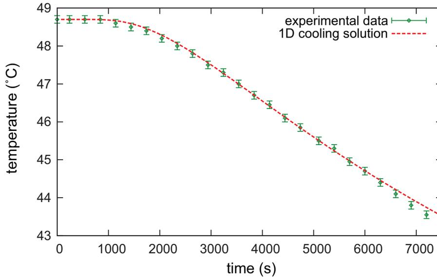
**Fig. 5.** The material thermal diffusivity is fitted against a 1-D cooling solution. The best fit provides a thermal diffusivity of  $2.8 \times 10^{-8} \text{ m}^2 \text{ s}^{-1}$ .
