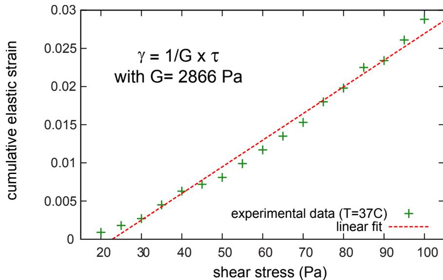
**Fig. 3.** Strain-stress curve obtained using the strain augmentation synchronous with the stress growth prior to reaching the plastic yield stress.
