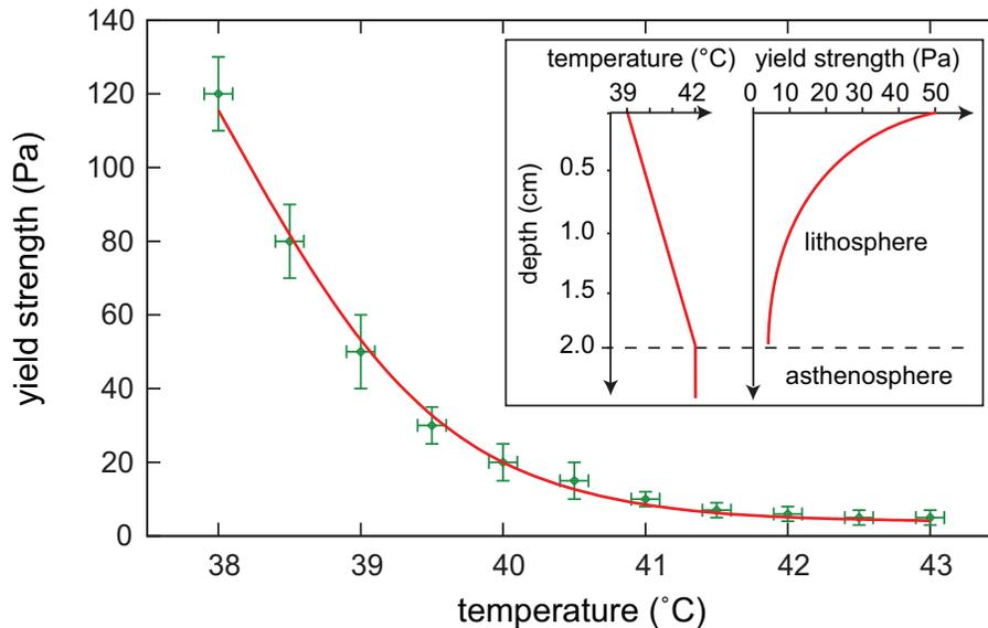
**Fig. 4.** Evolution of the plastic yield stress with temperature. The plastic yield stress decreases with increasing temperature. Inset: Once the temperature gradient in the model lithosphere is known, the experimental curve is used to draw the strength envelop of the model lithosphere prior to deformation.
