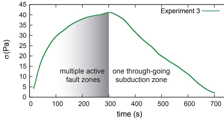
**Fig. 13.** Convergence parallel normal stress recorded in the back of the overriding plate in Experiment 3. The stress keeps increasing at the beginning of the experiment despite the formation of multiple shear zones. The stress decreases only once one shear zone becomes through-going. Strain is then localized into this zone (see Fig. 11b) and stress decreases.
