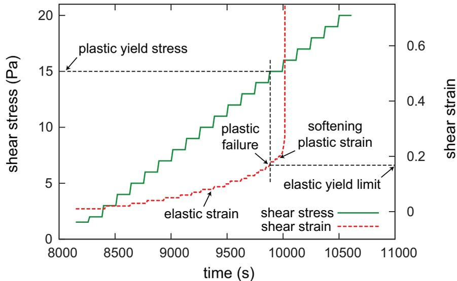
**Fig. 2.** Procedure employed to measure the materials mechanical properties. A constant shear stress is imposed on the sample during each time step, and then ramped up. For low stresses, the shear strain increases synchronously with the stress increase and then remains stable. When the plastic yield stress is reached the shear strain increases rapidly during the constant-stress creep step.
