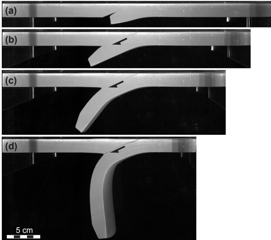
**Fig. 9.** Side images of the model in Experiment 2. The negative buoyancy of the subducted lithosphere tends to steepen the slab.
