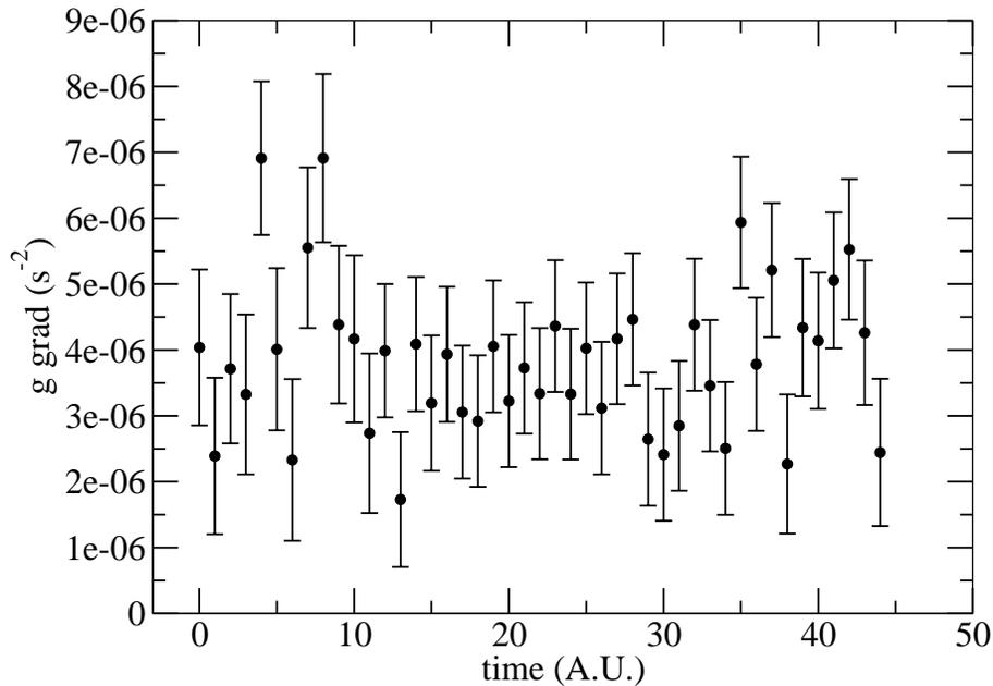
**Fig. 4.** Results of the best fit elaboration of the data provided by the FG5 gravimeter when installed in room 67. The best fit is used to obtain information on the gravity gradient at the FG5 site. We have grouped data from 50 drops (500 s time) in which we suppose both  $g$  and its gradient are constant. On x-axis there is the time after 10:20 UTC, 5 October, 2009 and the central part of the plot is during the night.
