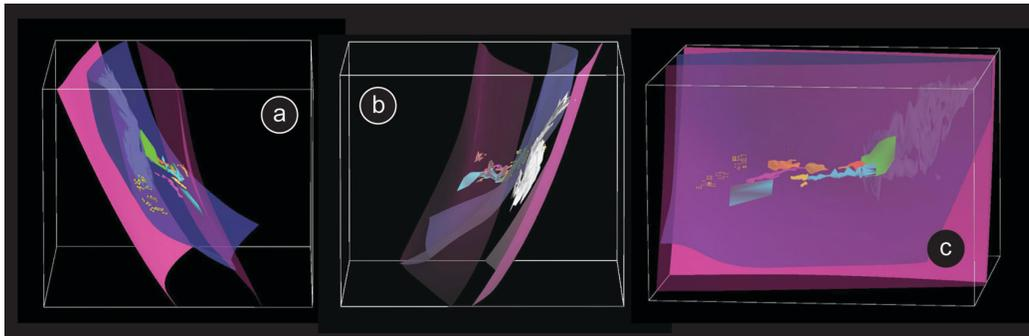
**Fig. 3.** Geometry of the Kristineberg deposit VMS lenses. **(a)** Cross-sectional view towards east. **(b)** Cross-sectional view towards west. **(c)** Longitudinal view towards north. Selected high-strain zones are shown for reference in different shades of magenta (see the Supplement for details). Height of the bounding boxes are 2.5 km.
