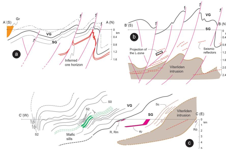
**Fig. 4.** Geological cross-sections, see Fig. 2a for location. **(a)** Cross-section through the contact zone between the metavolcanic and metasedimentary rocks, Gr = late-orogenic granite, **(b)** cross-section along the “high-resolution” seismic profile in Dehghannejad et al. (2010). See the Supplement for the location of L-zone. **(c)** Longitudinal E–W cross-section. Abbreviations for ore deposits as in Fig. 2.
