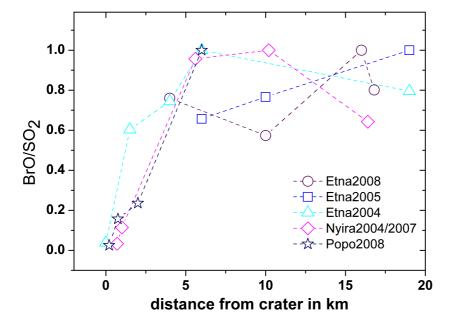
**Fig. 3.** BrO is formed by volcanic atmospheric-gas-interaction, but strong increase is (only) seen up to about 5 km (young plume of some minutes), BrO/SO<sub>2</sub> ratios seem to move into a plateau afterwards. The BrO/SO<sub>2</sub> ratios were normalised for a better comparison of the various sites. For more information see text.
