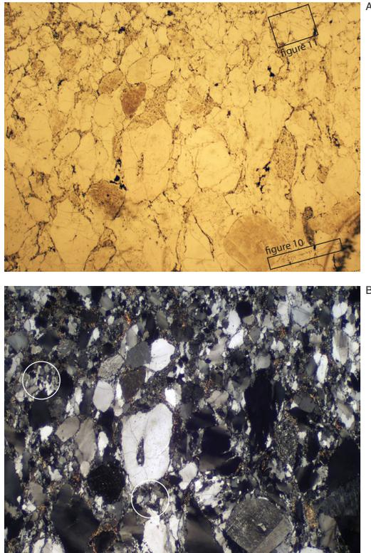
**Fig. 7.** Photomicrographs of sample 148d oriented with bedding horizontal and vertical tectonic foliation marked by preferred orientation of porphyroclasts and subgrains. **(A)** unpolarized. **(B)** Cross polarized. Locations of Figs. 10 and 11 are outlined in **(A)**. The white circles in **(B)** indicate two locations dominated by “midsized” recrystallized grains as discussed in the text. FOV ~ 7 mm.
