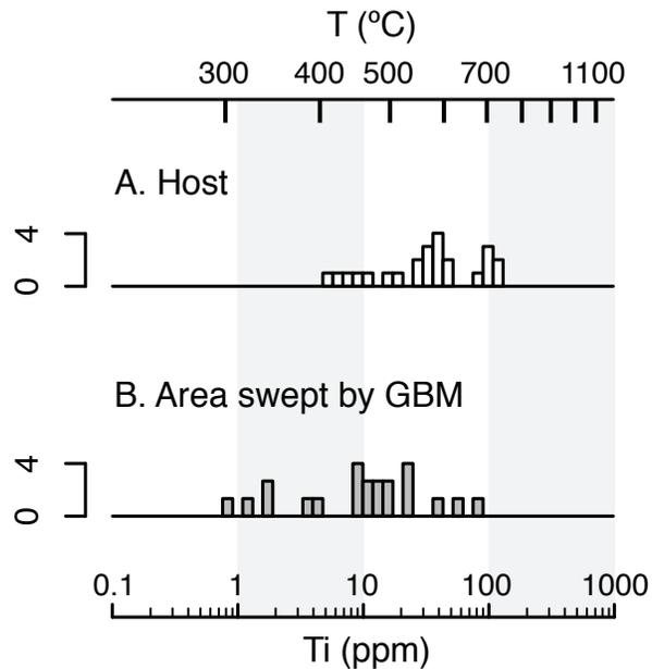
**Fig. 15.** Comparison of compiled Ti analyses in **(A)** six detrital porphyroclasts and **(B)** regions of the same porphyroclasts believed to have recrystallized due to grain boundary migration (GBM). An example of one such site is shown in Fig. 11. Temperature scale shown is based on Thomas et al. (2010) calibration assuming  $25^{\circ} \text{ km}^{-1}$ .
