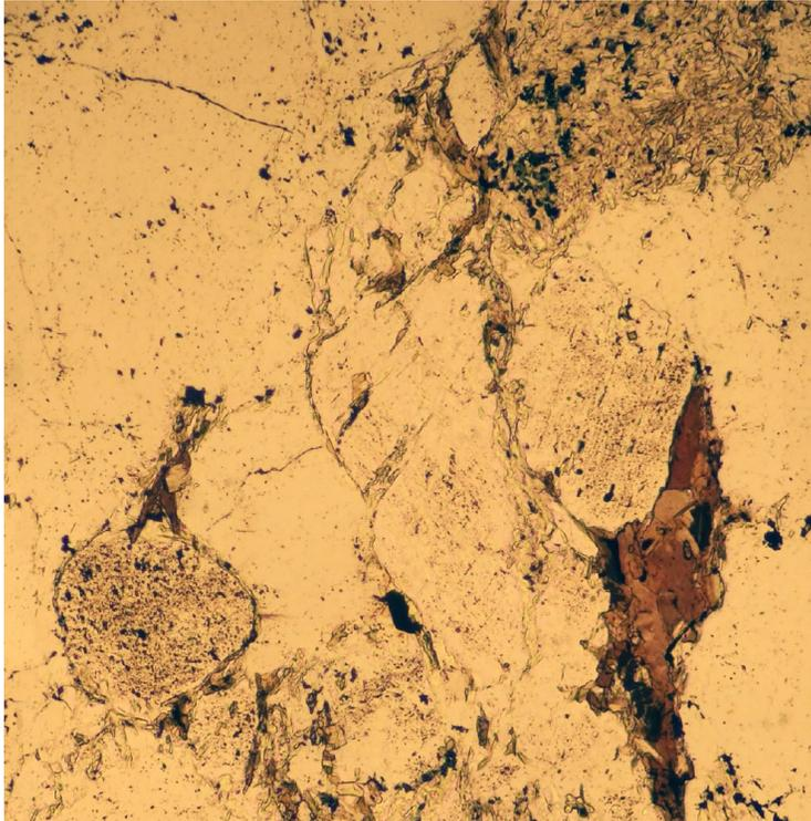
**Fig. 8.** Photomicrograph of sample 148d showing growth of metamorphic biotite in strain fringes on two detrital feldspar grains in the core of the Tachien anticline. Bedding and tectonic shortening direction (WNW-ESE) are horizontal in the figure. FOV 0.9 mm.
