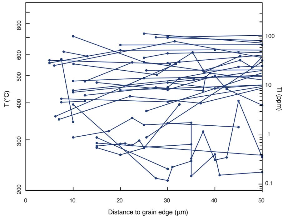
**Fig. 16.** Ti concentration vs. distance to grain edge in porphyroclasts.
