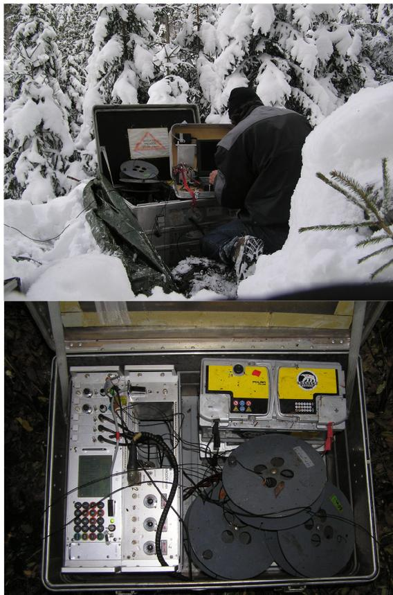
**Fig. D1.** Measuring device RAP (bottom) used in this study. Together with a triaxial fluxgate magnetometer and Ag–AgCl electrodes the equipment was developed at the University of Göttingen. Snow cover (top) showed to be advantageous to reduce temperature related noise.
