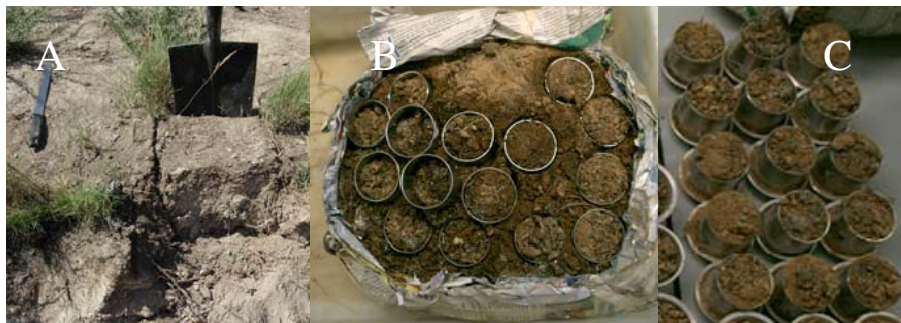
Fig. 1. Samples preparation: (A) block extraction, (B) subsamples of the blocks; and (C) subsamples preparation.
