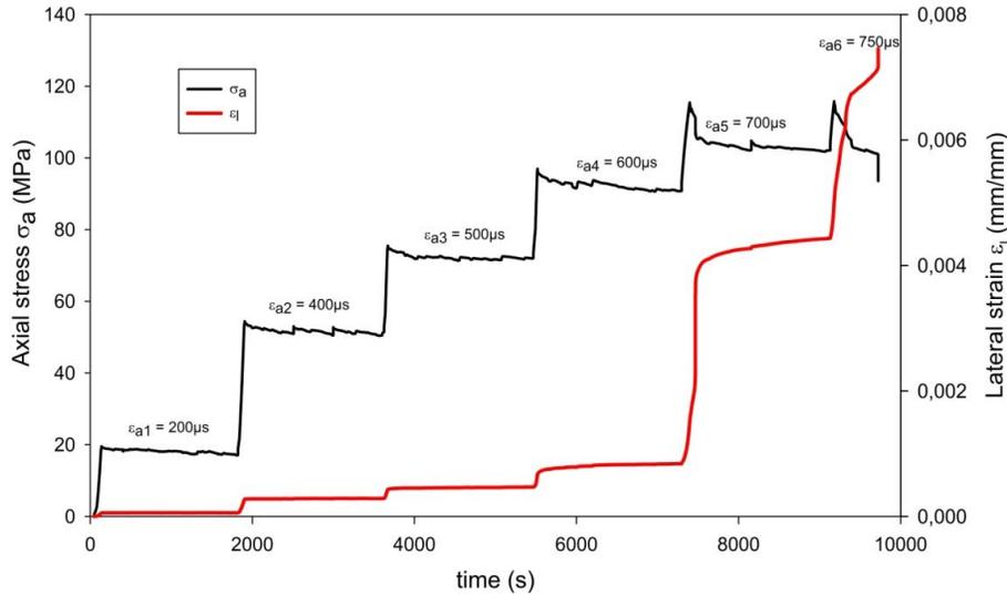
**Fig. 4.** Example of a 6-stage relaxation test on sandstone.
