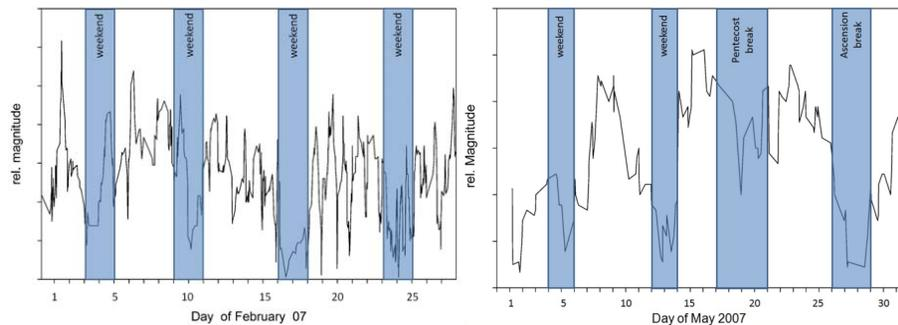
**Fig. 2.** (a) (left) Magnitudes of mining induced seismic events in February 2007) and (b), (right) May 2007. The plot line is a computed running average of 5 single magnitudes.
