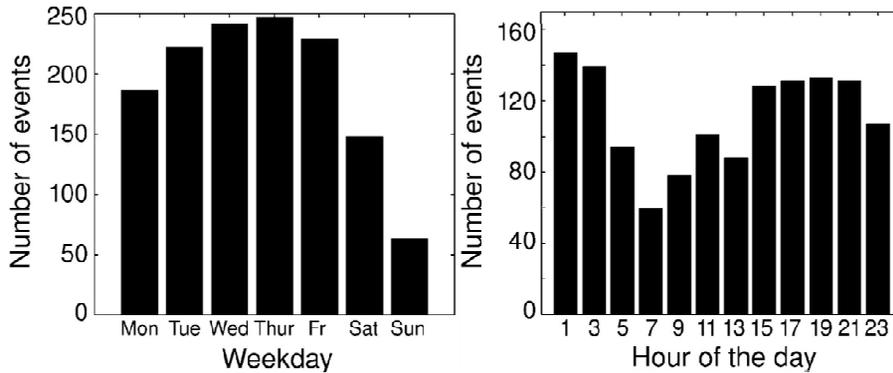
**Fig. 1. (a)** (left) Number of mining induced seismic events during a working week. **(b)** (right) Number of mining induced seismic events during a working day (Bischoff et al., 2010).
