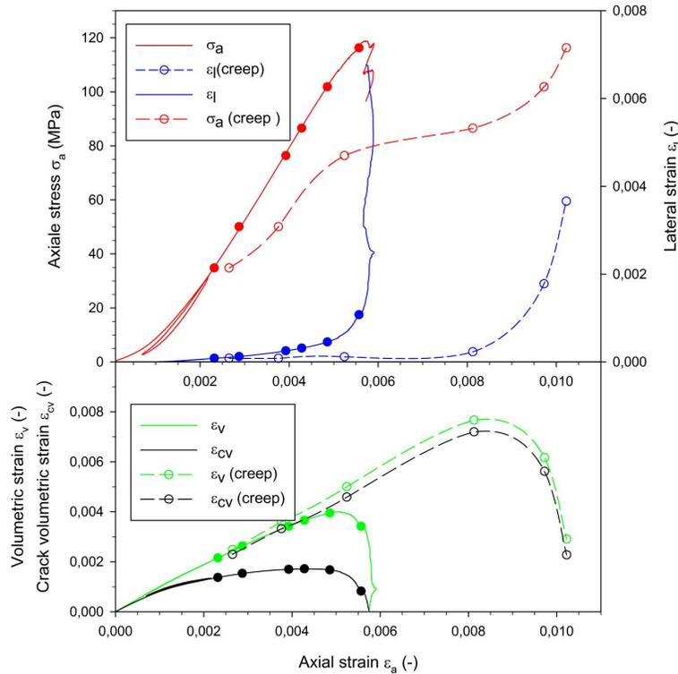
**Fig. 7.** Comprehensive graph showing stress-strain data of a UCS test (solid lines) and creep test (dashed lines) on sandstones from the same layer of the hanging wall in the mine.
