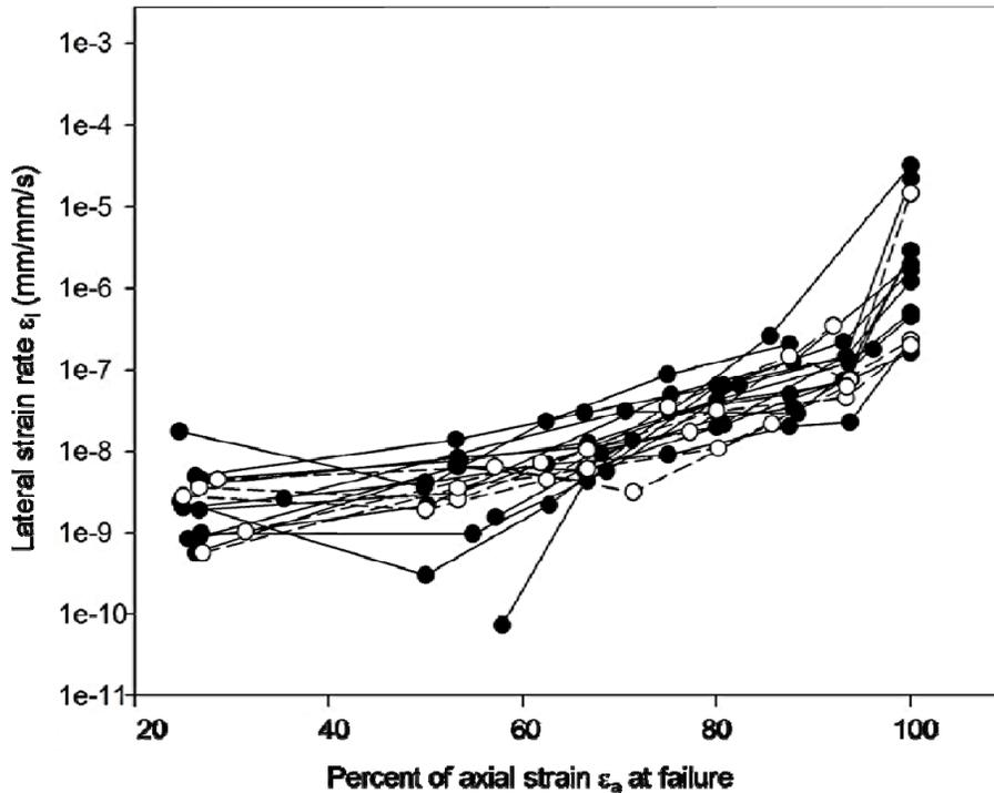
**Fig. 8.** Lateral strain rates as a function of axial strain levels for sandstone from the Ruhr mining district (Hellenkamp, 2011). Data from multistage creep tests on intact sandstones (black dots) and pre-damaged (open dots) sandstones from the mine.
