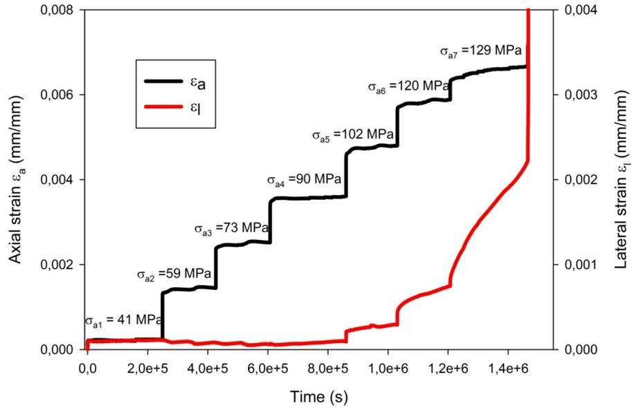
**Fig. 5.** Example of a multistage creep test on sandstone.
