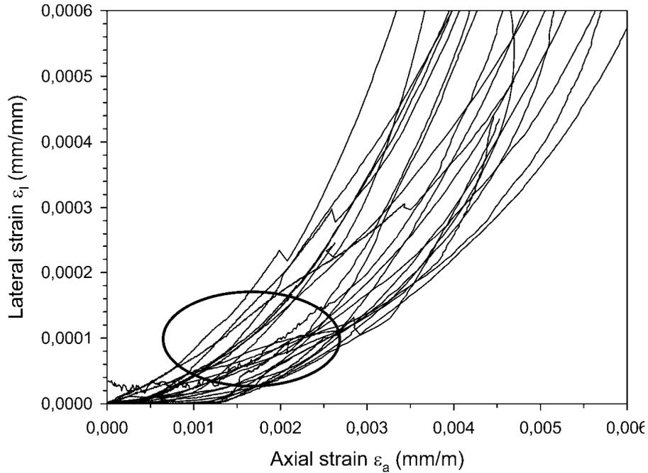
**Fig. 6.** Lateral vs. axial strain curves for estimating the critical extension strain.
