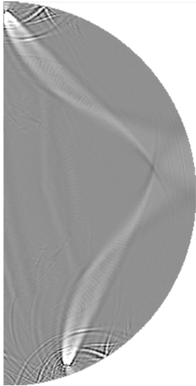
Figure 18. A snapshot of a time-dependent sensitivity kernel, denoting the “region of influence” in which this particular instance in the seismogram may “see” structure which deviates from the background model. The plot shows an instance within the PP surface multiple for P wavespeeds. Such kernels are not only the basis for waveform tomography, but may also aid in identifying obscure arrivals in the seismogram.
