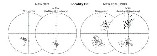
Fig. 6. Equal area projections of both in situ and tilt corrected ChRMs from our site OC (left) and from the same locality of Tozzi et al. (1988) (right), illustrating the apparent clockwise rotation that would result from a tilt correction of the bedding at this locality. The strata here have a primary dip (Fig. 7) and should be considered in in situ coordinates. Symbols are as in Fig. 5.
