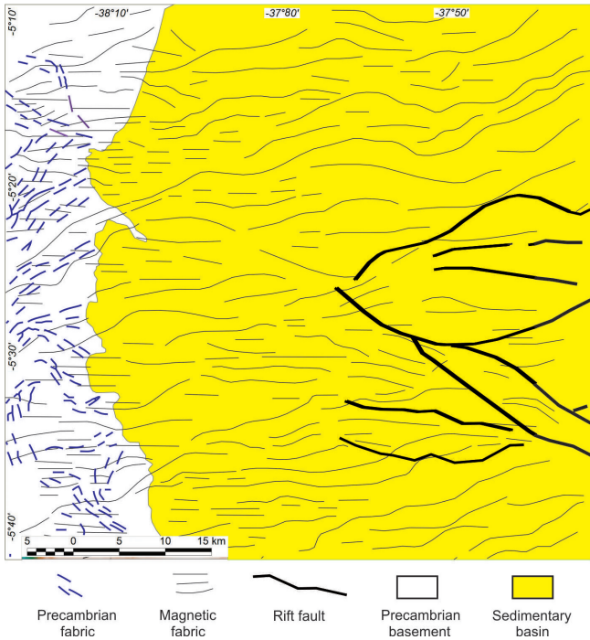
Figure 2908 Comparison between Precambrian structural fabric derived from remote sensing and NE-SW to E-W trending magnetic lineaments.
