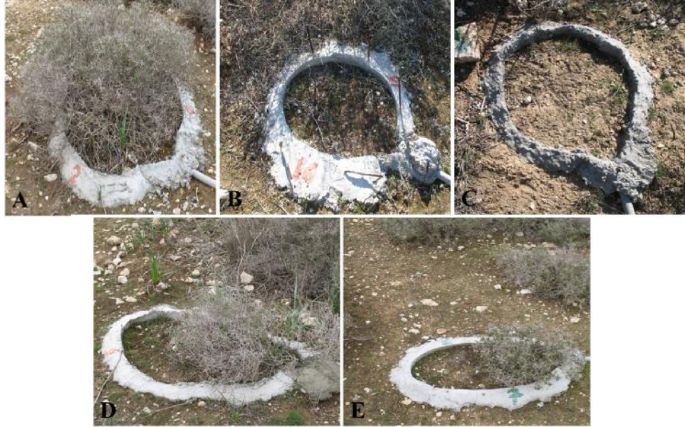
773 Fig. 3. Small runoff plots. A- Shrub (SH); B- Intershrub area (IS); C-Trampling route 774 (RU); D- Intershrub area + shrub ( ISSI ); E- Route + shrub ( RSSR ). (February 2008).
