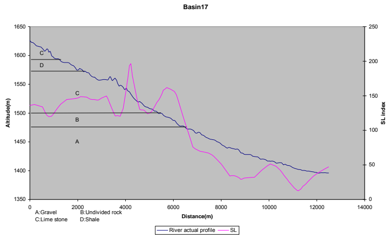
Figure 5 . Longitudinal river profiles and measured SL values for three subbasins in the study area.
