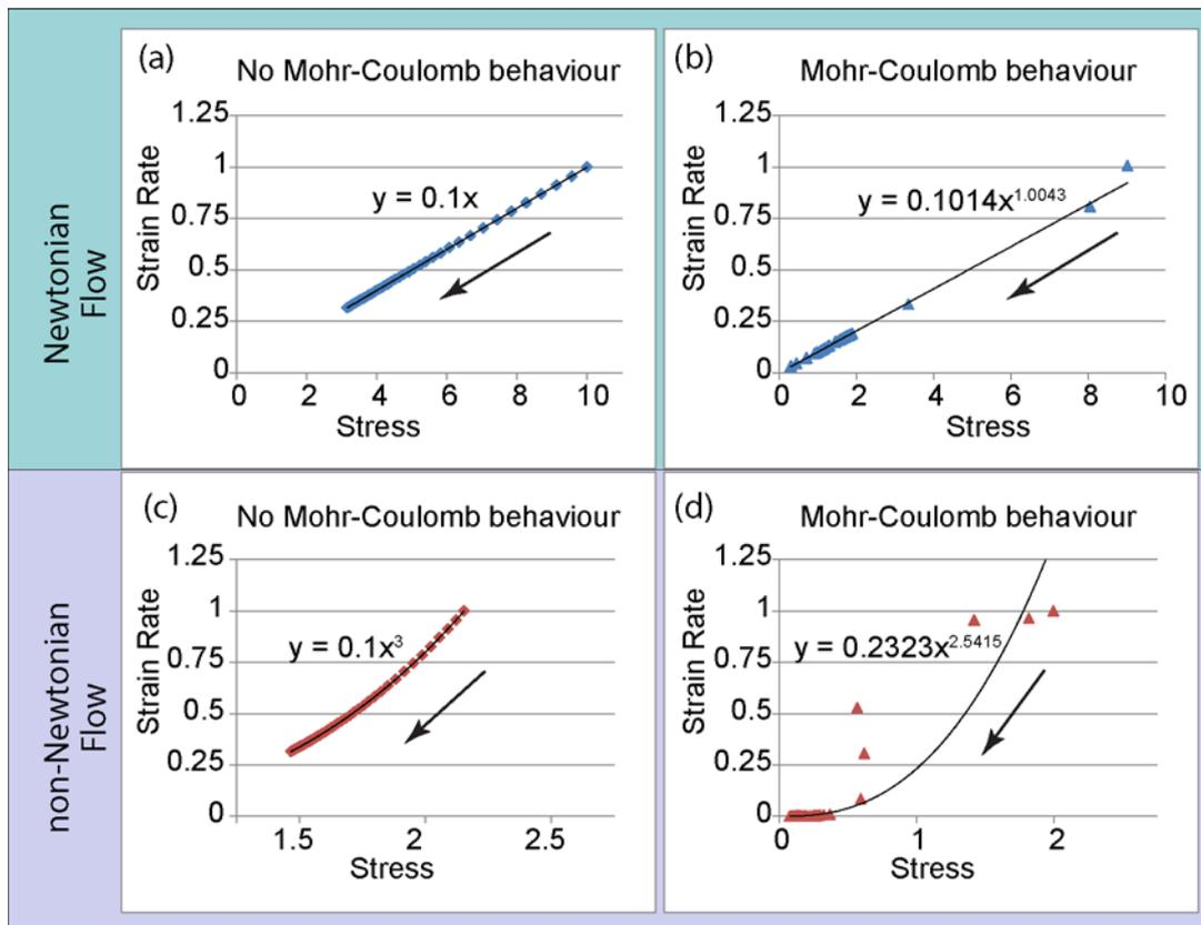
Figure S1: Graphs of Newtonian (a, b) and non-Newtonian (c, d) flow with Mohr-Coulomb brittle deformation behaviour (b and d) and with no Mohr-Coulomb behaviour (a, c). Relationship equations on (a) and (c) indicate Underworld is working as expected for Newtonian and non-Newtonian flow regimes. Black arrows indicate direction of simulation steps.
