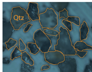
Figure 7. Photomicrographs by binocular microscope (reflected light) and by optical microscope (transmitted and reflected light) of the residue that remained in the reactor chamber after the experiment.
