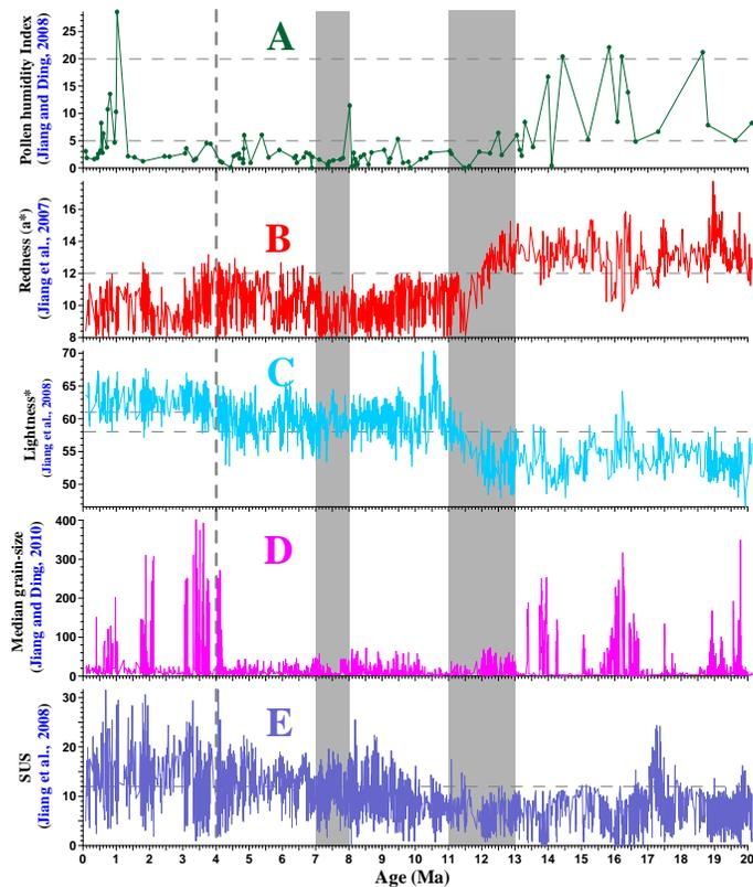
**Figure 4.** Comparison of **(a)** pollen humidity index (Jiang and Ding, 2008), **(b)** redness ( $a^*$ , Jiang et al., 2007), **(c)** lightness ( $L^*$ , Jiang et al., 2008), **(d)** median grain-size (Md, Jiang and Ding, 2010), and **(e)** susceptibility (SUS, Jiang et al., 2008) from the Sikouzi section at Guyuan, Ningxia Province, China.
