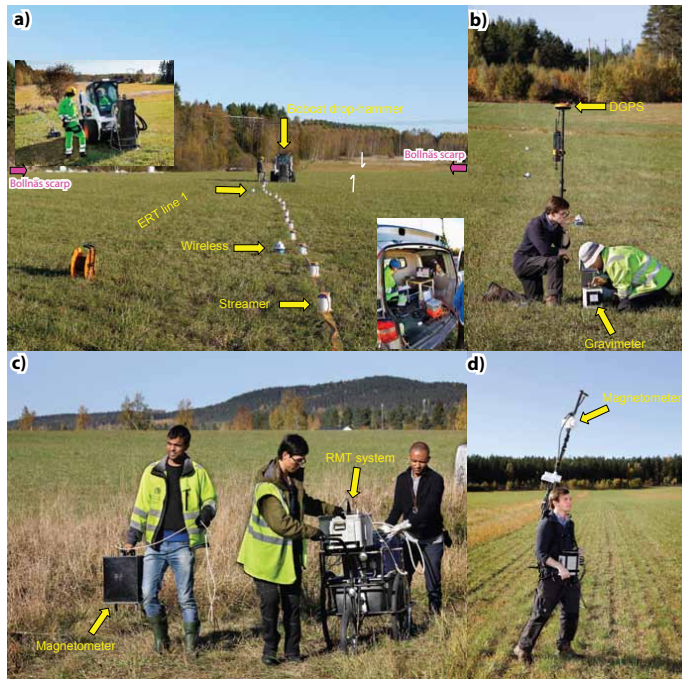
Figure 4. (a) Field photos showing (a) the seismic data acquisition using combined wireless (24-fixed, 20 m spacing) and cabled (92-MEMs-based streamer and planted, 2–4 m spacing) seismic recorders and Bobcat-mounted drop hammer as the seismic source. (b) Gravity (128 points were measured) and geodetic surveying. (c) RMT data acquisition (10 m spacing along profiles 1 and 2). (d) Total-field magnetic surveying. The geophysical data acquisition took totally 6 days in two separate field campaigns during October 2014. The Bollnäs scarp and its apparent displacement is visible in (a; see the half arrows).
