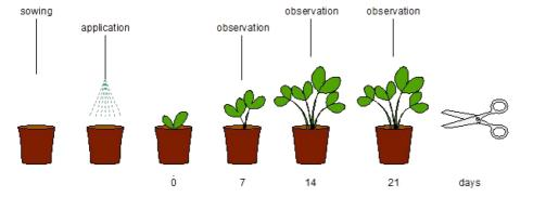
Figure 2. Layout of the phytotoxicity test.
