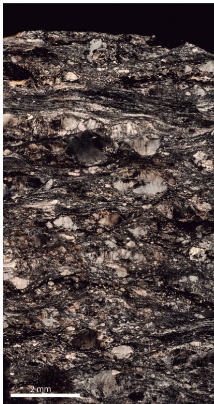
Figure 3. Cross-polarized optical micrograph showing the microstructure of sample PE19 from the Pernambuco shear zone. K-feldspar porphyroclasts (domain 1) alternate with monomineralic quartz veins (domain 2). Dark layers of ultrafine-grained feldspathic mixture form an anastomosing network wrapping the porphyroclasts, and are particularly well developed in a C' orientation consistent with the sinistral sense of shear (domain 3). See text for further explanations.
