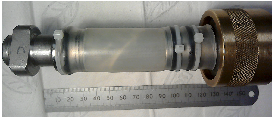
Figure 3. A jacketed sample with a 45° pre-cut. Around the sample is a 3 mm wall-thickness soft silicone rubber sleeve to minimise the risk of the sliding parts puncturing the outer jacket that seals against ingress of confining pressure fluid. On the left is the bayonet connector that allows samples to be tested in uniaxially-symmetric extension. 1 cm scale divisions.
