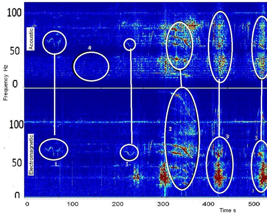
**Figure 2.** An example of spectrochronogram for lithosphere acoustic (top) and electromagnetic (bottom) signal variations. They are connected by vertical lines on the figure. Indications of the lithospherics correspond to their types.
