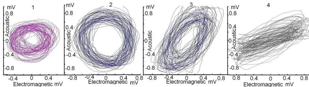
**Figure 4.** Phase relations of anomalies of different acoustic and electromagnetic signals (Lissajous figures). In horizontal direction is the electromagnetic signal amplitude. In vertical direction is the acoustic signal amplitude. 1 – “monosigmoid”, 2 – “polysigmoid”, 3 – “trill”, 4 – “roar”.
