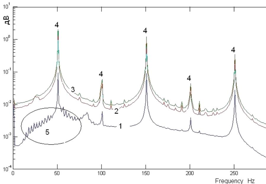
**Figure 1.** Averaged spectra of initial signals. 1 – acoustic signal spectrum; 2 – noise signal spectrum; 3 – mixture signal spectrum; 4 – industrial noise frequencies; 5 – borehole acoustic resonances.
