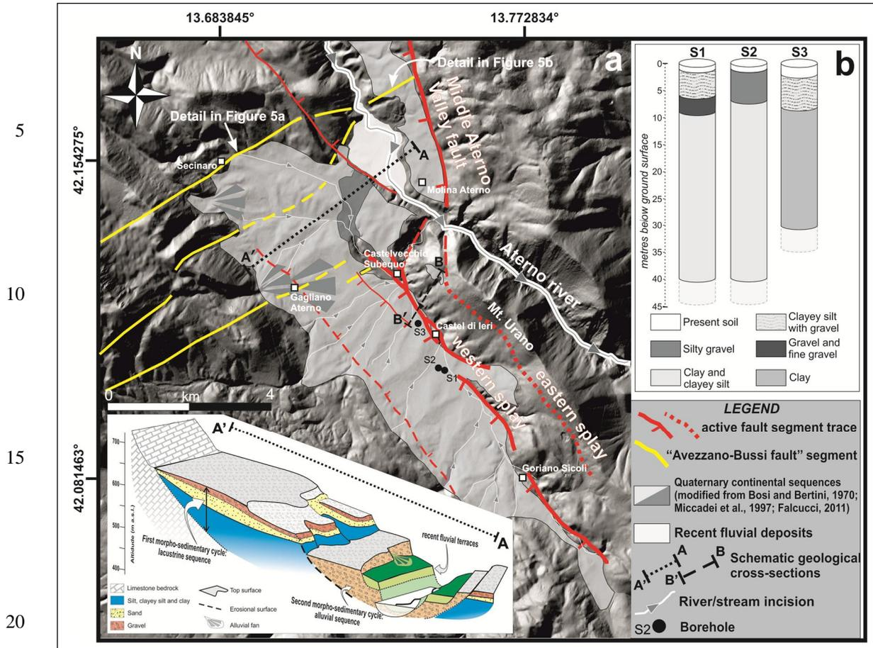
Figure 2: a) Shaded relief of the Subequana Valley (plan view) on which simplified geological map (modified after Bosi and Bertini, 1970; Miccadei et al., 1997; Falcucci, 2011) is reported; morpho-stratigraphic reconstruction of the Quaternary succession of the Subequana Valley, inset. b) Stratigraphy of boreholes drilled in the Subequana Valley during the seventies of the past century.
