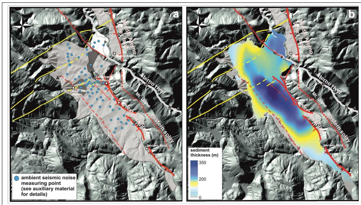
**Figure 7:** a) Simplified geological map of the Subequana Valley (legend as in figure 2); location of the ambient seismic noise measuring points, blue circles. b) Reconstruction of the deep geometry of the Subequana Valley (legend as in figure 2), defined by the sedimentary fill thickness.
