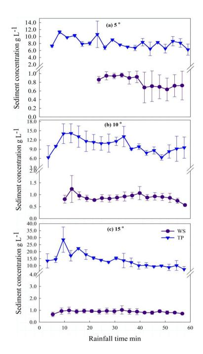
Figure 5 Runoff rates versus sediment concentrations for WS and TP management treatment.
