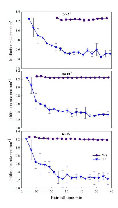
Figure 4 Dynamics of the Sc in WS and TP plot during the simulated rainfall event.
