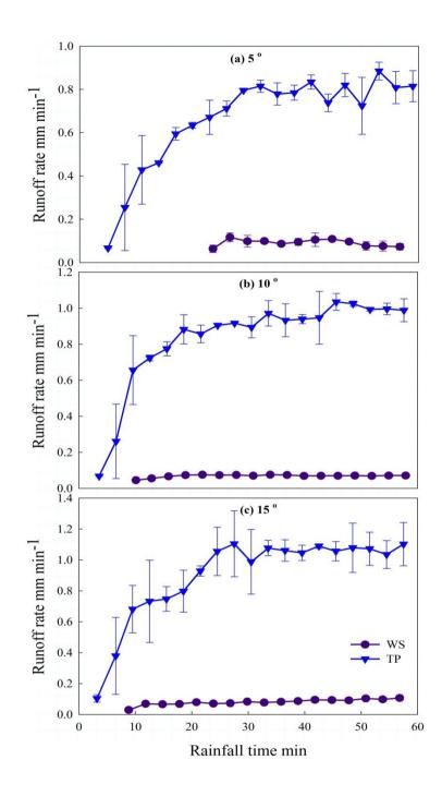
Figure 3 Dynamics of the infiltration rate in WS and TP plot during the simulated rainfall event.
