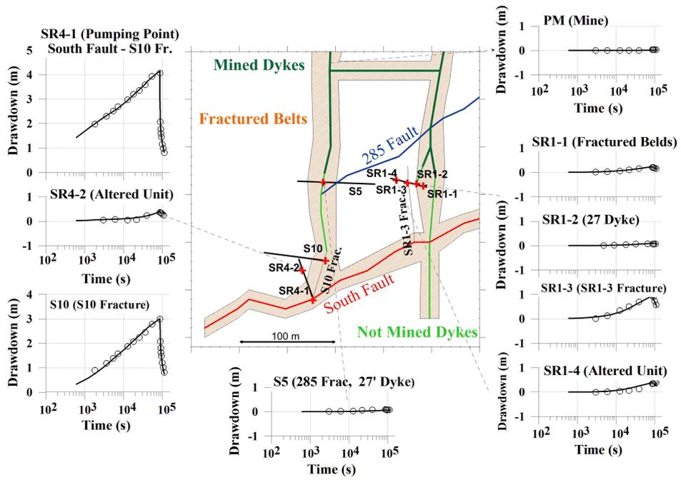
**Fig. 1.** Figure 9: Results obtained after calibrating the SR4-1 cross-hole test are indicated by a black line, observed data are indicated with circles using a 3D model. All graphs maintain the vertical scale
