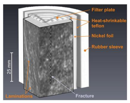
Figure 3: The Computed tomography (CT) image of the rock sample with a rescaled voxel dimension  $(0.25 \times 0.25 \times 0.25 \text{ mm}^3)$ . The upper filter plate, the units of the core-holder and lamination of the sample are highlighted in orange. The fracture is indicated by a dotted purple line.
