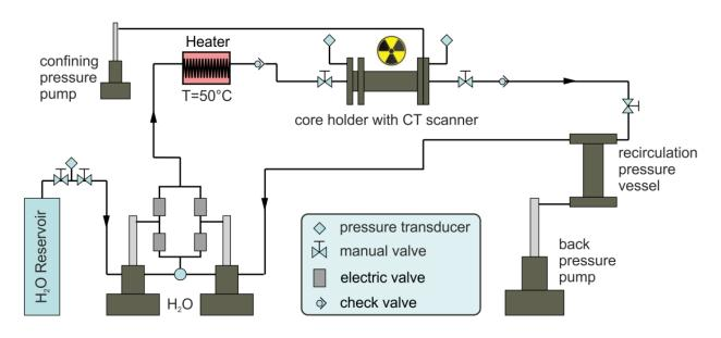
Figure 2: Schematic setup of the core-flooding apparatus for single-phase (H<sub>2</sub>O) flow experiments (after Huo and Benson, 2015).
