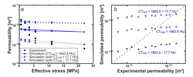
Figure 7: (a) Measured and simulated permeabilities of the entire core-sample versus effective stress. Simulation results are obtained by forward modelling (cf. Eq.3) and by changing  $CT_{mat}$  according to the mean standard deviation of the CT measurements (cf. Eq.7) and (b) corresponding deviations between experimental and simulated permeabilities indicating a systematic error.
