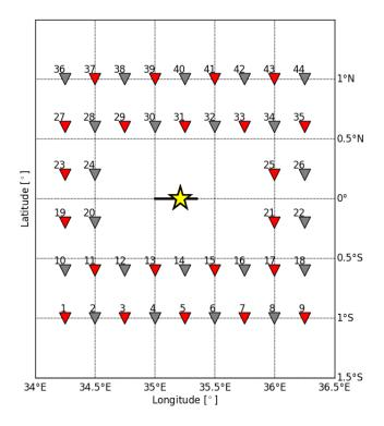
Figure 1. 44 receivers, marked as grey (only used without rotation data) and red triangles (used for all inversions) are setup around the source with a spacing of  $0.4^{\circ}$  latitude and  $0.25^{\circ}$  longitude. The fault is illustrated as a black line with constant latitude of  $0^{\circ}$ . The yellow star marks the epicenter of the earthquake.
