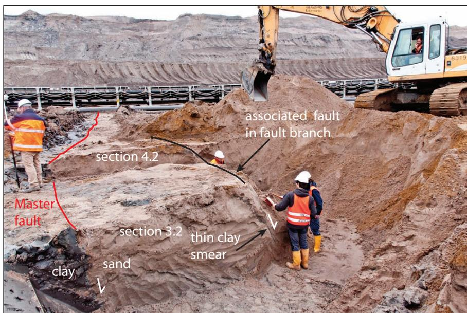
**Figure 3.** Overview showing the excavation side. The master fault is depicted in red, while a black line shows the associated synthetic fault at which the clay smears were excavated. Trenches 3 and 4 are visible.
