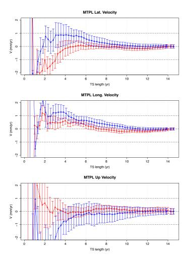
Figure 3: Velocity convergence for the station MTPL for the forward (red) and backward (blue) analyses.
