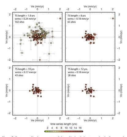
Figure 7: East versus North components of the residuals relative to a regional reference, color-coded based on the time series lengths.
