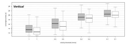
Figure 4: Whisker plots of convergence time for four velocity thresholds (1.0, 0.5, 0.2, and 0.1 mm/yr). Thick bars, boxes, and dashed bars represent the median, quartile (25% and 75%) and extreme values of the distributions for the 44 stations with at least 10 years of data. Grey and white whisker plots correspond to unfiltered (raw) and filtered (with common-mode correction) data.
