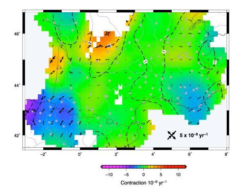
Figure 8: Smoothed horizontal strain rate field for the Western Alps and Pyrenees region. Dashed lines are strain rate standard error.
