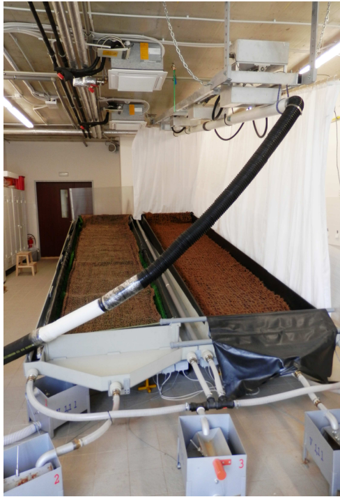
Fig. 1. Norton Ladder Rainfall Simulator above test beds with mechanical toggle flow metres. C400 coir erosion control net spread in the test bed.
