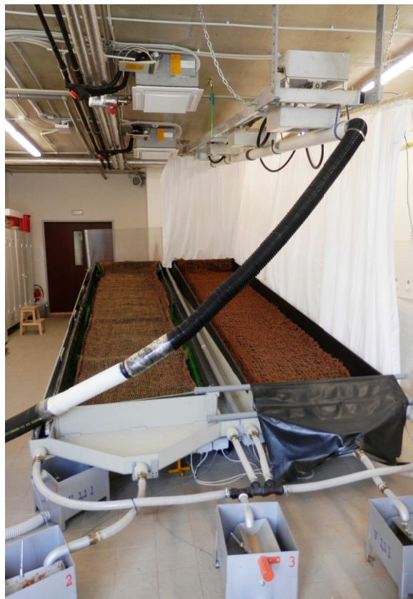
Fig. 1. Norton Ladder Rainfall Simulator above test beds with mechanical toggle flow metres. C400 coir erosion control net spread in the test bed.
