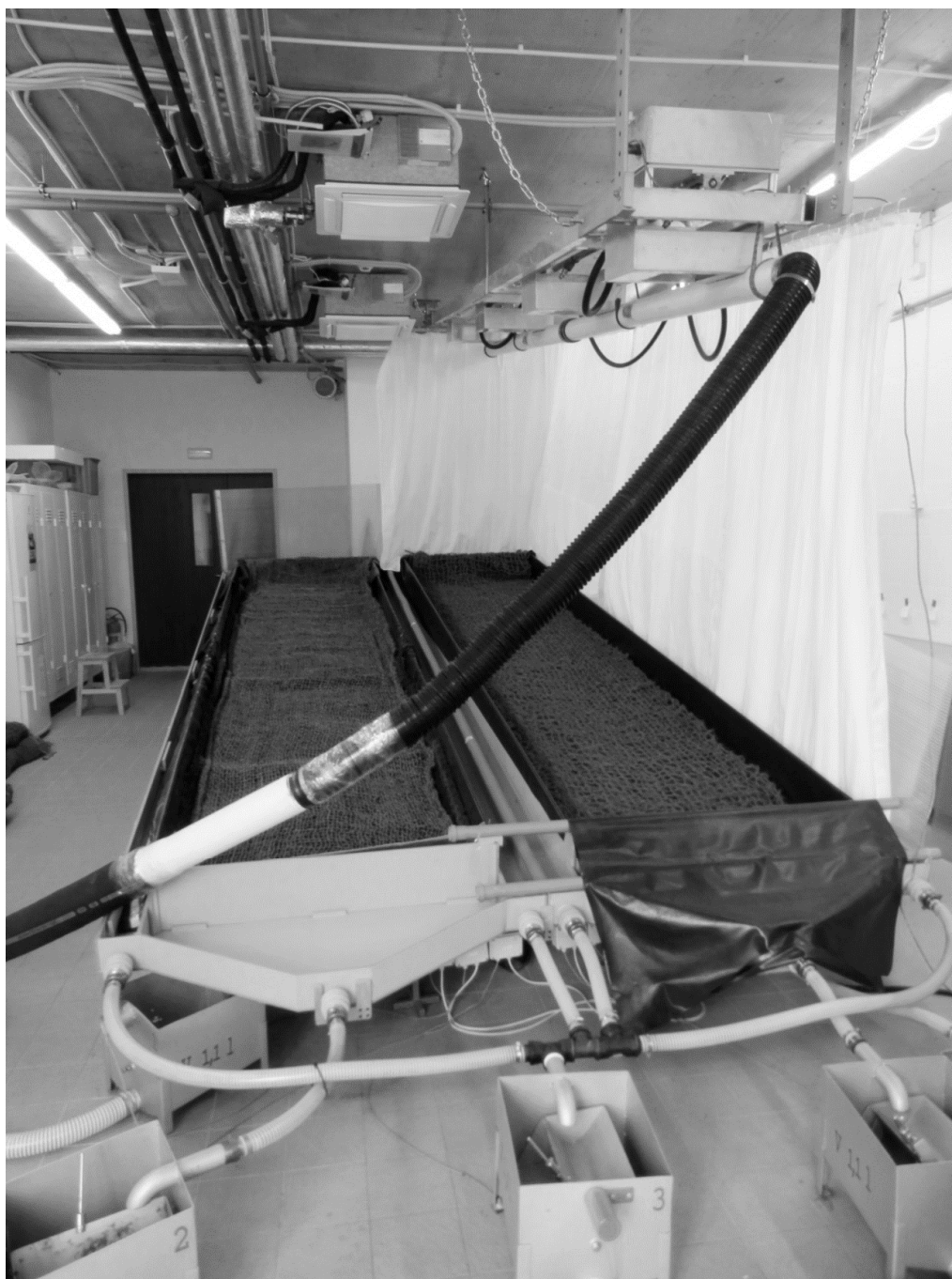
Figure 1 Norton Ladder Rainfall Simulator above test beds with mechanical toggle flow metres. C400 coir erosion control net spread in the test bed.
