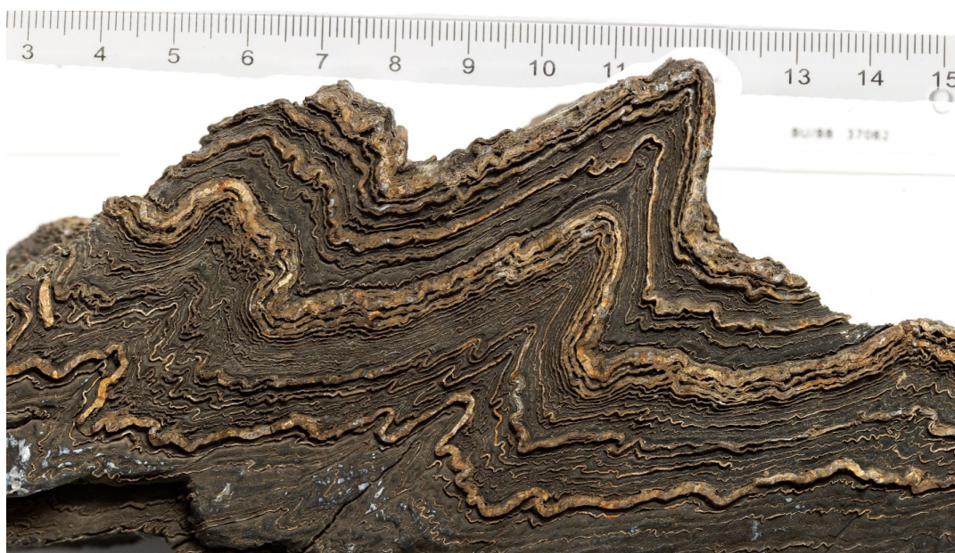
Figure 10. Multilayer folds showing that the size of individual folds (quantified by amplitude and distance between hinges) is related to their layer thickness and that folds become systematically smaller as their layer thickness becomes thinner. Carbonates with silicate-rich layers belonging to the Jurassic El Quemado formation. The sample was found by Stéphane Leresche around the Mount Fitz Roy, Southern Patagonia, and the photo was made by Yoann Jaquet.
