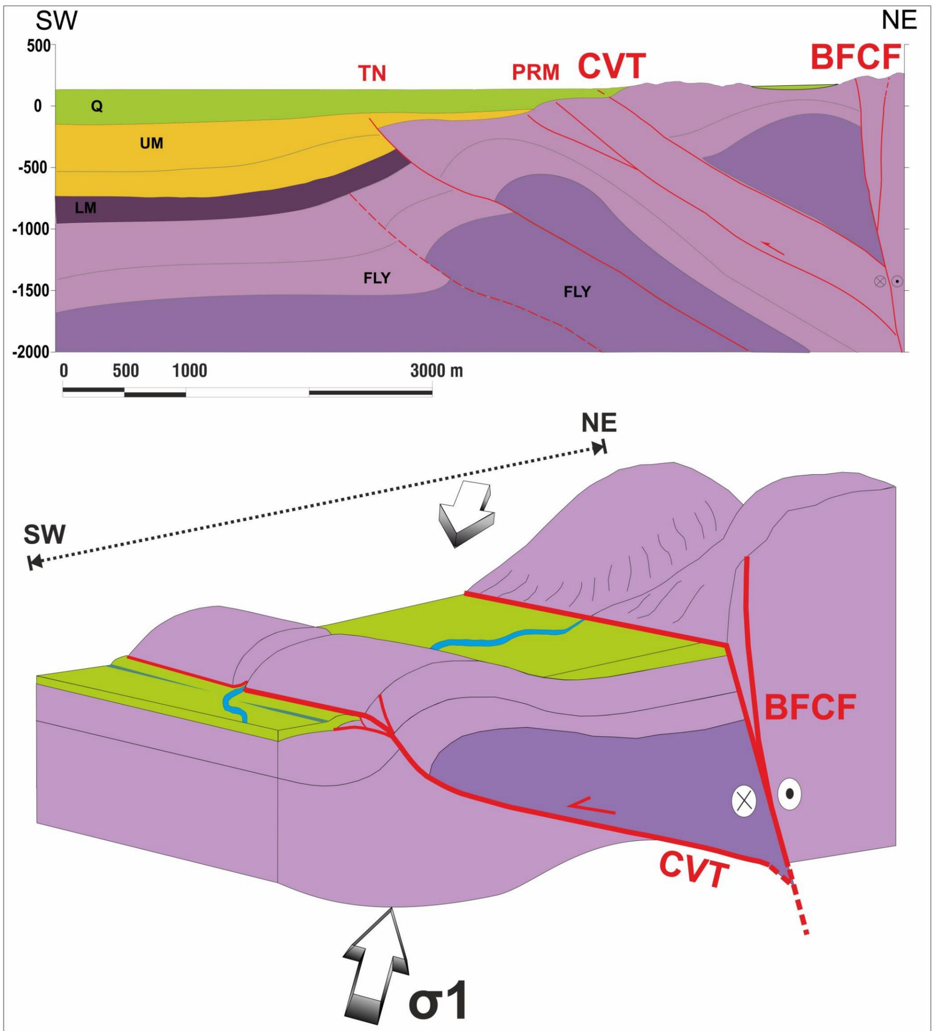
Figure 7: Geological cross section based on the seismic line of Figure 2 (AA' in Figure 1b) and 3-D scheme (lower panel) of the BFCF-CVT system. Q: Quaternary; UM: Middle-Upper Miocene Molasse; LM: Cavanella Group (Lower-Middle Miocene); FLY: Upper Cretaceous – Lower Eocene turbiditic sequence. TN: Tarnovo Nappe front (according to Placer et al., 2010)
