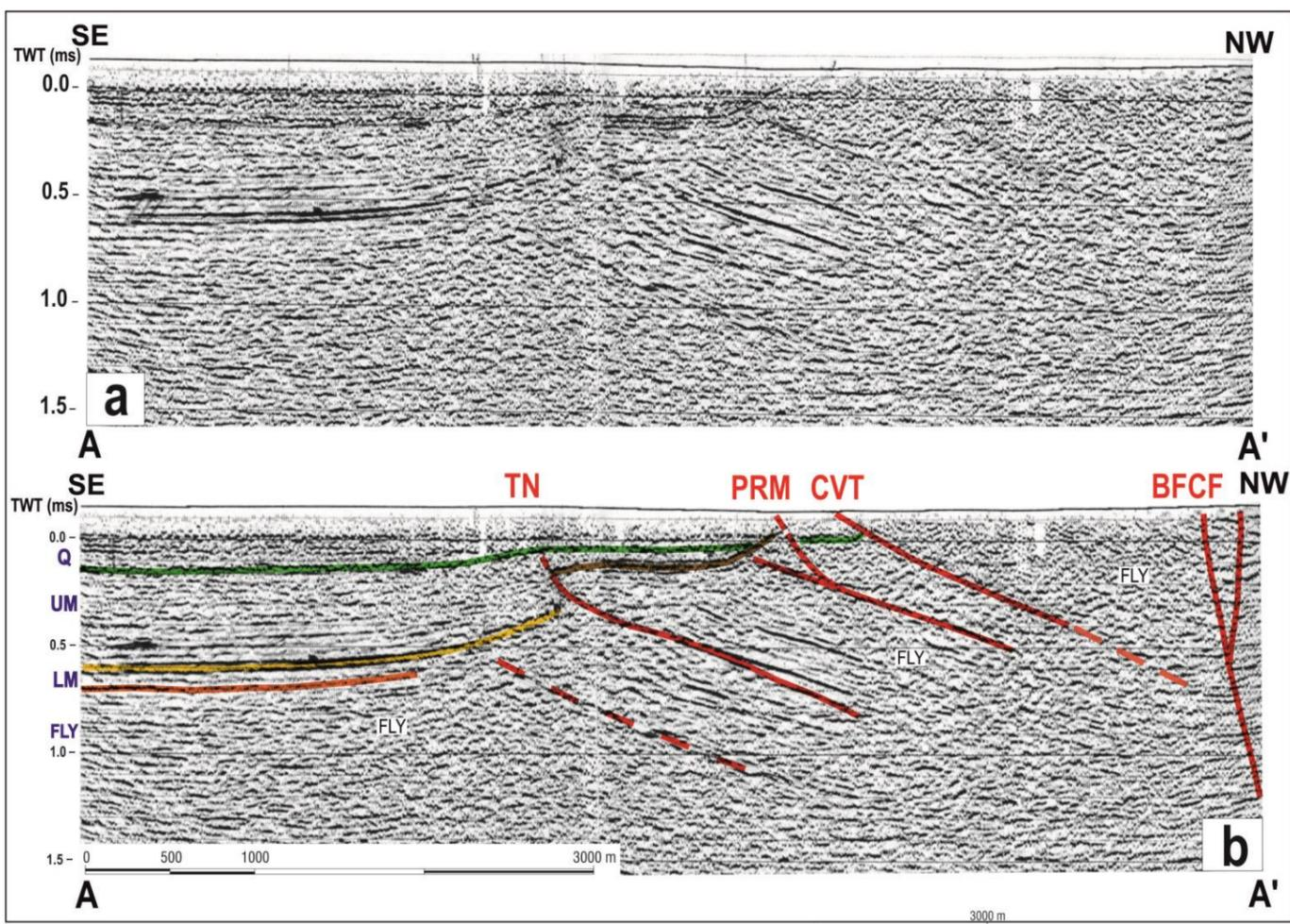
Figure 2: a) Reflection seismic section crossing the study area; b) Interpretation (line drawing) of the reflection seismic section (A-A' in Fig. 1b). Q: Quaternary; UM: Middle-Upper Miocene Molasse; LM: Cavanella Group (Lower-Middle Miocene); FLY: Upper Cretaceous-Lower Eocene p.p. turbiditic units.
