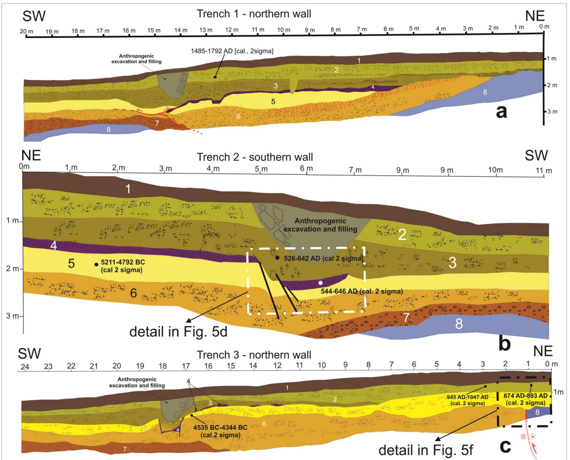
Figure 6: Trench walls, stratigraphic schemes. Units: 1, soil; 2, 3, 5 and 6, colluvial deposits; 4 and 7, fluvial deposits; 8, turbiditic bedrock.
