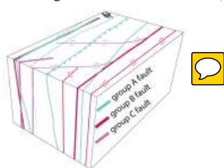
Figure 2. Schematic bloc diagram showing geometrical relationships between faults of different orientation groups (modified after Wehrens et al. 2017).
