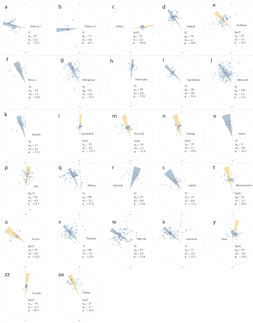
Figure 6: Locality results from sedimentary basins (Ulukışla and Sivas basins, and basins overlying the Tauride fold-and-thrust belt). Equal area projections of ChRM directions and their means with associated error ellipses (DD 95 , DI 95 ) according to (Deenen et al., 2011), either before (orange; NoTC) or after tectonic correction (blue; TC). Rejected directions (after 45° cut-off) are displayed in grey, positive (negative) inclinations are shown as solid (open) circles. All directions have been converted to normal polarity (see also Table 1 ).
