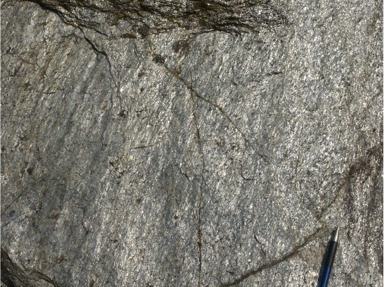
Figure S1: Outcrop of sample FG1315. The shiny aspect on the XY plane is due to white mica. The stretching lineation is marked by the alignment of white mica and quartz.
