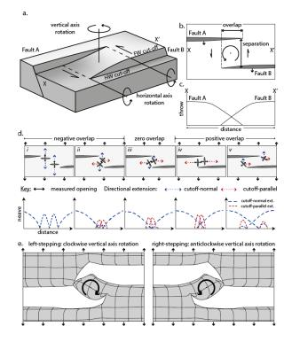
**Figure 1.** (a) Schematic diagram illustrating a relay zone between two normal faults (after Ferrill and Morris, 2001); (b) Map view of the block model in (a) showing fault overlap and separation; (c) Distance versus displacement (throw) profile for transect X-X'; (di-v) Second-order fault geometries as a function of fault overlap (redrawn from Tentler and Acocella, 2010)
