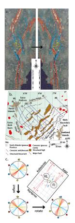
**Figure 10.** (a) Reflection of left-stepping Krafla faults to a right-stepping NE Atlantic rift configuration; (b) Map of the European margin of the NE Atlantic showing the broad NE-SW basin trend. JL: Judd Lineament; CL: Clare Lineament; GKL: Grimur Kamban Lineament; VL: Victory Lineament; EL: Erlend Lineament; ML: Møre Lineament; BL: Brynhild
