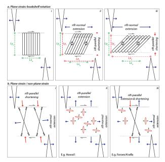
**Figure 6.** Horizontal plane 2D conceptual models for inter-fault/inter-rift relay rotation. (a) Bookshelf rotation model showing (i-iii) progressive rotation leading to rift normal extension, and rift-parallel shortening; (b) Schematic models for structures observed in the study areas presented here: (i) conjugate extensional shear faults, (ii) extension fractures, and (iii)
