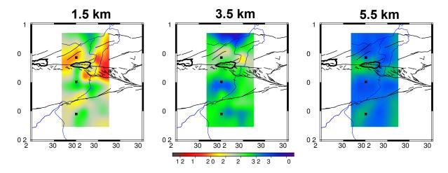
**Figure 6.** Isotropic S-wave velocity maps at 1.5, 3.5 and 5.5 km depth. Black lines show the mapped faults. The blue line represents the Sakarya River, flowing towards the north. The black squares represent the locations of the nodes shown in Fig. 5.
