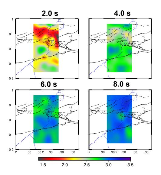
**Figure 3.** Rayleigh wave phase velocity maps at 2.0 to 8.0 s period. Black lines show the mapped faults. The blue line represents the Sakarya River, flowing towards the north.
