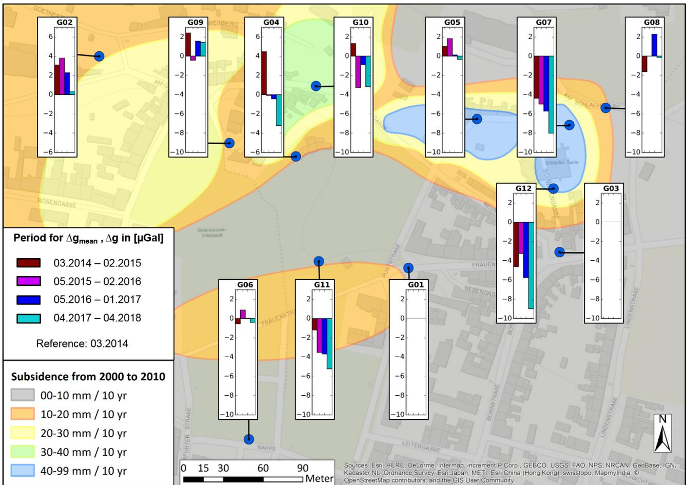
**Figure 10.** Temporal variations of mean gravity observations  $\Delta g_{\text{mean}}$  over each year of data, referenced to March 2014, on the points of the gravity network (blue dots). The gravity values for each survey point are derived from least squares adjustments assuming that G01 and G03 are stable over time. The adjusted gravity differences are hydrologically corrected for soil water content applying an individual regression coefficient for each gravity difference.
