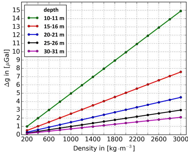
**Figure 11.** Expected changes in gravity against density for a 1 m thick layer located beneath a survey point and at different depths, with a spatial dimension of  $dx = 10$  m,  $dy = 10$  m, and  $dz = 1$  m.
